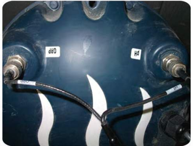
Connect the wires from the ORP probe to the genertor. Make sure the label on the cord matches the label on the generator
