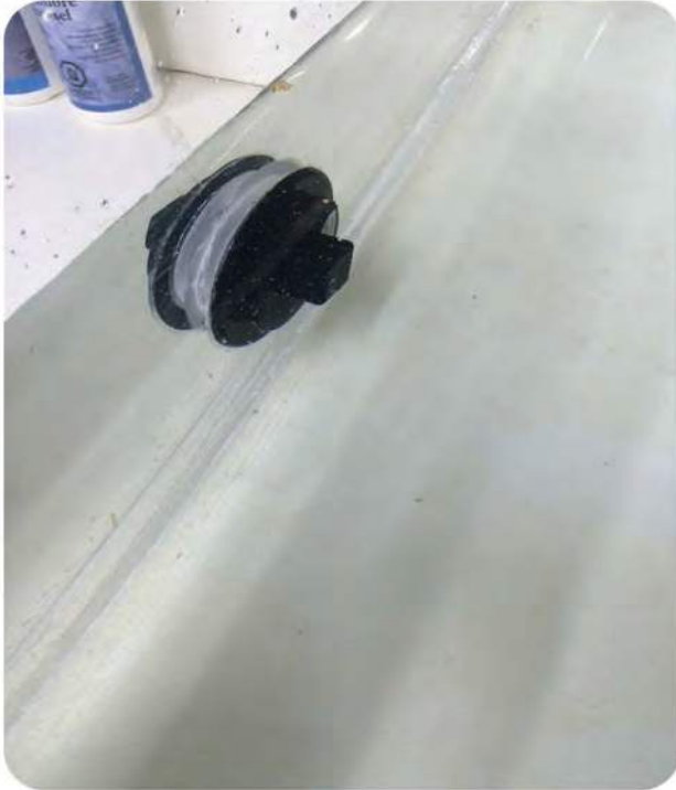
Fill water to just above the ORP Probe wall fitting
