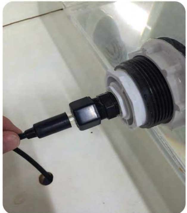
Insert probe into strain relief
