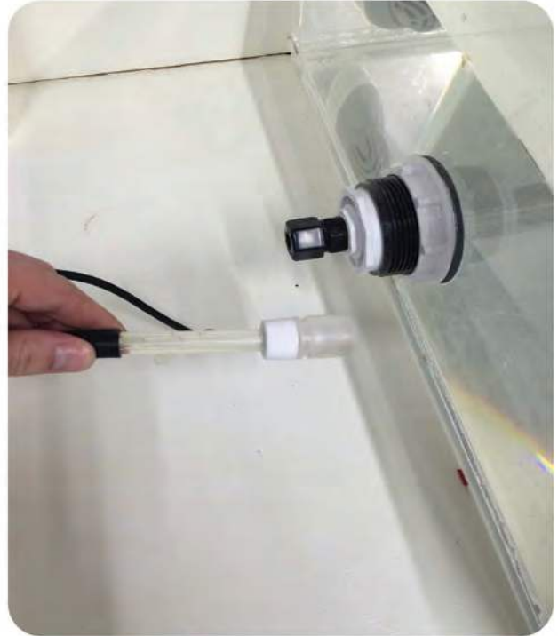
Get Probe ready to install. The Probe needs to stay in its solution until you are ready to install.
