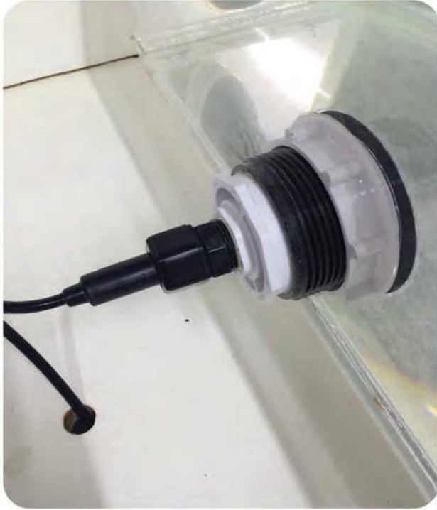
Tighten strain relief until tight
